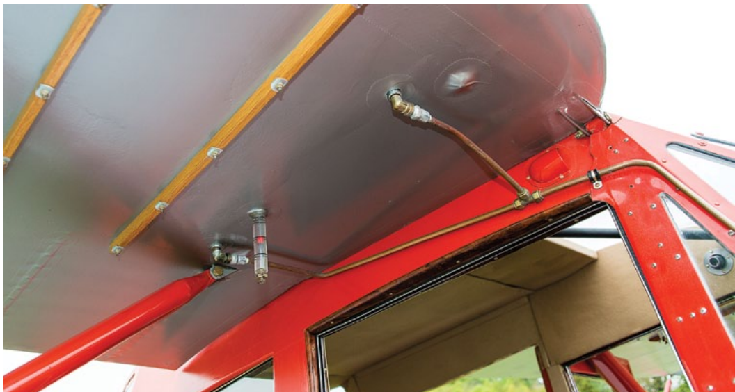
Above The view from the back seat is better than from the front. David Keays shows how it’s done... Right Steps are essential for refuelling and the total capacity is a generous 66 gallons Bottom right The overstamped model type indicates the change from OEC to UEC engine spec Below Outdoor plumbing – fuel pipes route outside the airframe and the sight gauge is easily visible through the wind-down window Left The WACO’s interplane struts are substantial, and pitot/static connections add a little extra drag
