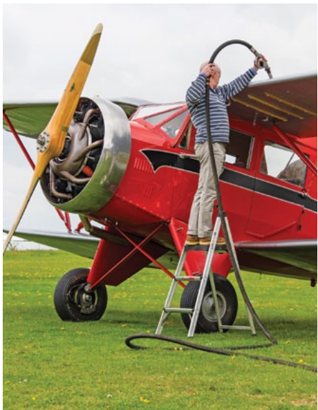
Above The view from the back seat is better than from the front. David Keays shows how it’s done... Right Steps are essential for refuelling and the total capacity is a generous 66 gallons Bottom right The overstamped model type indicates the change from OEC to UEC engine spec Below Outdoor plumbing – fuel pipes route outside the airframe and the sight gauge is easily visible through the wind-down window Left The WACO’s interplane struts are substantial, and pitot/static connections add a little extra drag
